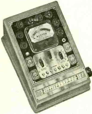
Model 773, at left, for combination with 772 Analyzer, or, at right, as individual portable unit.
